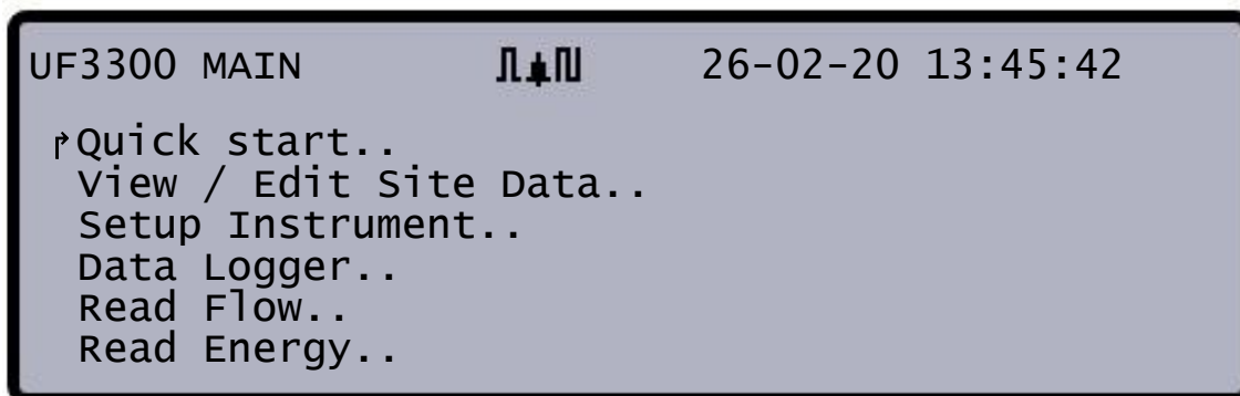
Figure 6 Main menu ( Read Energy and Data Logger options available with heat meter versions only)
