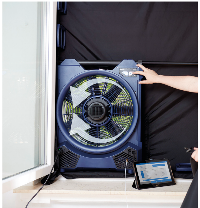
Standard-compliant Blower Door Measurement Measuring method according to ISO 9972, EN 13829 and common country-specific standards. Under- and overpressure measurement with flow rates up to 6000 m 3 /h without having to turn the fan unit.
