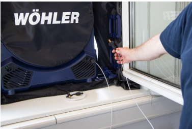
Fig. 20: The capillary tube is routed outdoors through the panel
