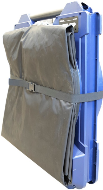
Fig. 23: Panel secured to the blower fan by the lashing belt for transport
