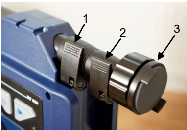
Fig. 14: Close-up view of the telescopic rod with clamps (1) and (2) as well as the head (3)
