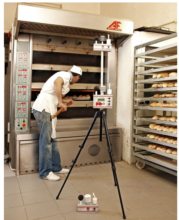
Three levels WBGT on the same vertical
