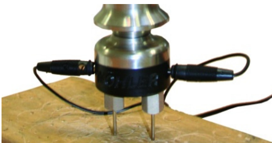
Fig. 9: Connecting the cable to the Wood Moisture Probe
