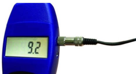
Fig. 10: Connecting the cable to the Wöhler HBF 420
