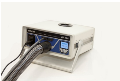
Fig. 17: Hoses and cable connected to the measuring instrument for the leakage test class N: Mains cable, pressure hose and plastic hose
