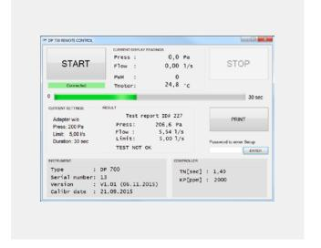
Leakage tests on several 100 m² of installed ductwork systems.
