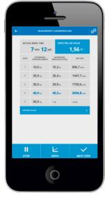
The Wöhler BC 600 automatically performs the complete series of measurements according to DIN EN ISO 9972/DIN EN 13829.
