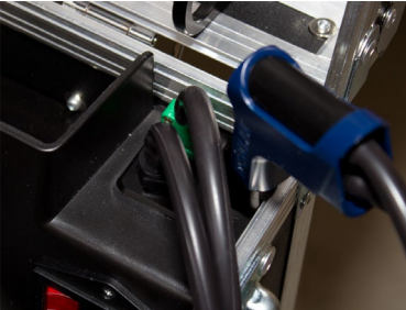
Fig. 12: Connecting the probe and cable-hose assembly
