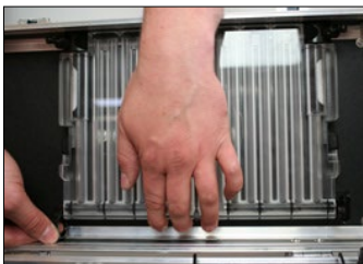
Fig. 65: Refitting the condenser
