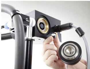
Fig. 77: Removing the filter cartridge
