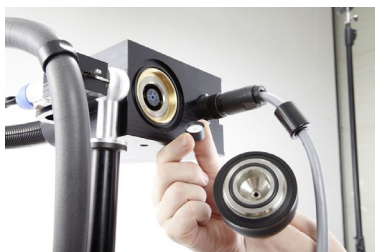
Fig. 9: Changing the filter
