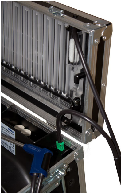
Probe and cable-hose assembly connection for flue gas analysis
