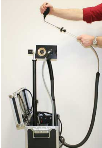
Fig. 72: Purging the sampling probe, the hose and the digital mass scale unit
