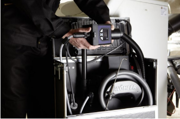
Fig. 4: Extending the telescopic stand
