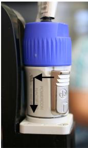
Fig. 88: Inserting the connector plug
