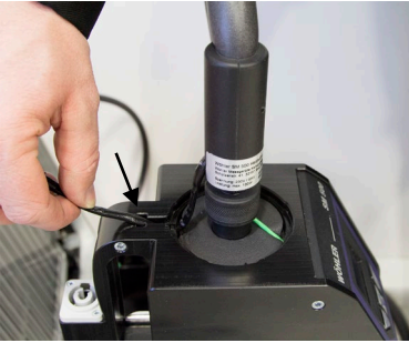
Fig. 89: Indentation for the connection cable of the heated sample intake hose
