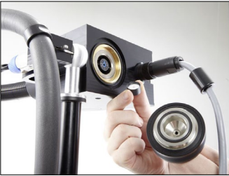
Fig. 68: Inserting a used filter cartridge
