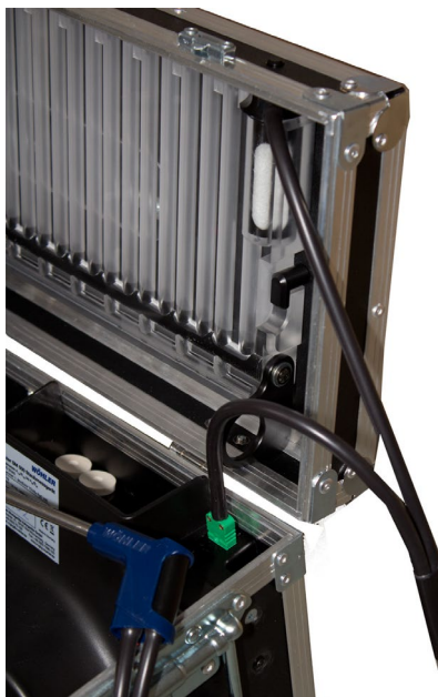
Fig. 13: Connection for flue gas analysis (special circumstances!)
