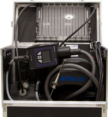
Fig. 15: Intake hose coiled around the reel
