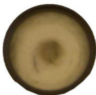
Fig. 10: Filter cartridge visibly loaded
