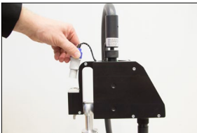
Fig. 83: Removing the connector plug
