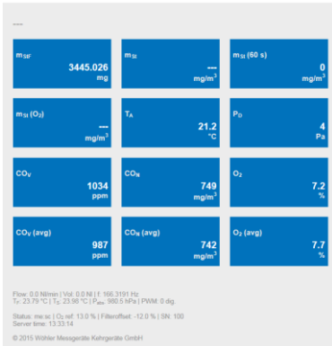
Fig. 27: Measurement data Messdaten Wöhler SM 500 displayed on the PC or mobile device.
