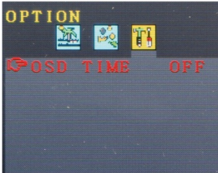
Fig. 13: automatic shutdown deactivated
