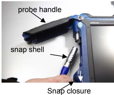
Fig. 24: Wöhler A 550 with open probe compartment
