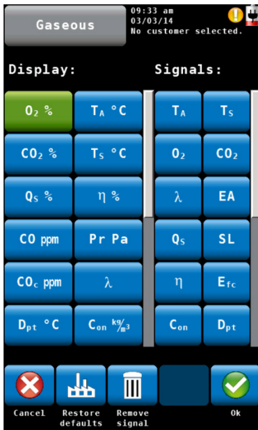
Fig. 58: Configuration of the readings segment.
