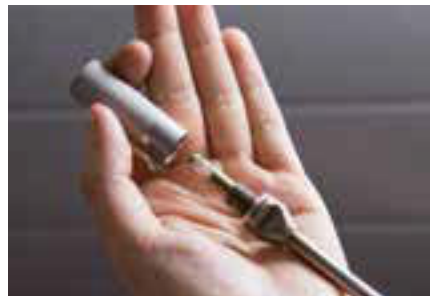
Sinter-filter probe removes dust (> 20 micron) from the sample gas to protect the analyzer against heavy dust loads
