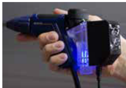
Battery-driven peltier cooler removes condensate from the sample gas for accurate NOx and SOx measurements
