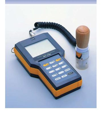
MT-900 supersedes the conventional MT-700 model. We have provided two new calibration curves under the labels "Broadleaf" and "Conifer", and by using these curves, it is possible to cover a wide moisture range - 6-80% (Broad-leaf) and 7-80% (Conifer). It is also possible to call up the calibration curves of the original 16 tree species. Furthermore, we have provided a printer output terminal so that data can be printed out by connecting to an optional printer.
